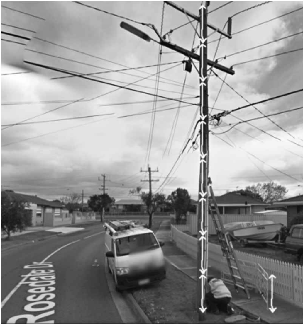
Figure 5: Google Street View image of the street containing the electricity poles near the plane's shadow, showing how to estimate the height of the pole. Source: Google maps.
